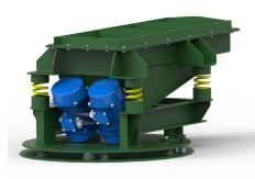
Electromechanical feeders are powered by twin rotary electric vibrators which provide a broader range of stroke/frequency combinations. Their flexibility is further enhanced with a variable frequency drive (VFD), which provides quick and easy adjustment without having to manually adjust the eccentric weights.
